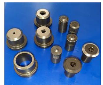
*Dies and punches for circular holes and valve holes*
